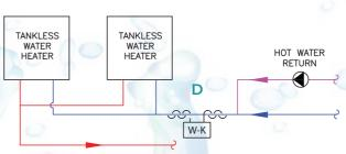
**E** For **Re-Circulating Systems** where water in constantly circulated, such as swimming pools, the Water-King should be fitted downstream of the pump, as close as possible to where the heating process is occurring.
