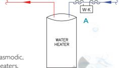
A Where point-of-use electric water heaters are installed and hot water demand is spasmodic, such as in an office, it's best to fit a dedicated unit to each water heater or cluster of heaters.
